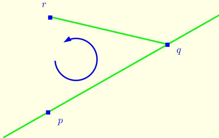
$$\begin{aligned} \text{orientation}(p, q, r) &= \text{sign} \left( \det \begin{bmatrix} p_x & p_y & 1 \\ q_x & q_y & 1 \\ r_x & r_y & 1 \end{bmatrix} \right) \\ &= \text{sign}((q_x - p_x)(r_y - p_y) - (q_y - p_y)(r_x - p_x)) \end{aligned}$$
